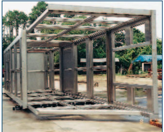
*Fig. 1 — The completed stainless steel elevator hoist. (Photos courtesy of Unlimited Welding Inc., Winter Springs, Fla.)*
