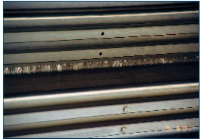
Fig. 3 — View of the FCAW-G weld deposit.
