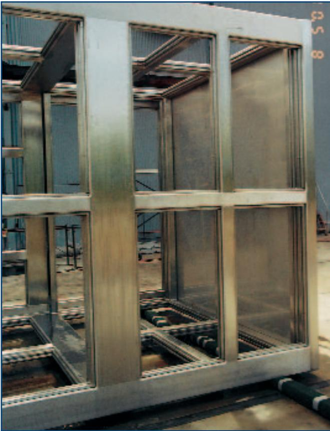
Fig. 2 — A view of the required No. 4 Satin finish weld surface.
